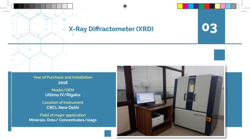
X-ray Diffractometer (XRD) is used to determine the atomic and molecular structure of a crystal/ powder, in which the crystalline structure causes a beam of incident X-rays to diffract into specific directions. By measuring the angles and intensity of these diffracted beams, identification of the minerals is carried out.
