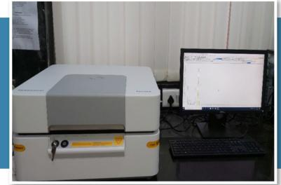
X-ray Fluorescence (XRF) is an analytical technique that uses the interaction of x-rays with a material to determine its elemental composition. XRF is suitable for analysis of solids, liquids and powders. It is a non-destructive analytical technique.
