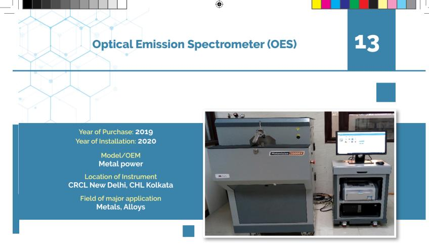
Optical Emission Spectroscopy (OES), is a well trusted and widely used analytical technique used to determine the elemental composition of a broad range of metals. The type of samples which can be tested using OES include samples of tubes, bolts, rods, wires, plates and many more.
