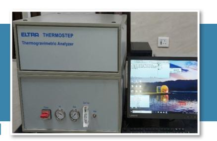
Thermogravimetry (TGA) is a technique that measures the change in weight of a sample as it is heated, cooled or held at constant temperature. Its main use is to characterize materials with regard to their composition. Application areas include plastics, elastomers and thermosets, mineral compounds etc.
