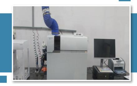
Inductively coupled plasma mass spectrometry (ICP-MS) atomizes the sample and creates atomic and small polyatomic ions, which are then detected by mass spectrometer. It can detect metals and several non-metals at very low concentrations i.e. PPB (Parts Per Billion). It can also detect different isotopes of the same element. It is used for simultaneous determination of elements in one test.
