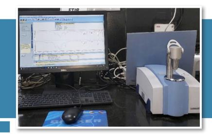
Identification of polymers and organic compounds in short time (01 minutes) is done by FTIR. This instrument can analyze above materials/substances in solid/liquid state.
