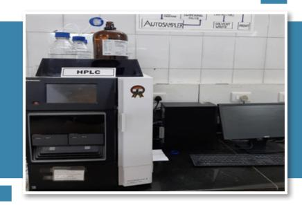
High-performance liquid chromatography (HPLC) is used to separate, identify, and quantify each constituent of a mixture of organic compounds. Availability of HPLC has enabled some of the Revenue Laboratories to obtain NABL accreditation for testing of azo dyes.
