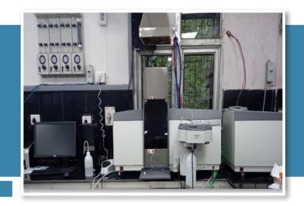
Atomic Absorption Spectrometry (AAS) is an analytical technique that measures the concentrations of elements. The technique makes use of the wavelengths of light specifically absorbed by an element. Concentration of elements is measured at ppm (parts per million) levels.
