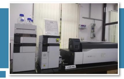
Liquid Chromatography with tandem mass spectrometry (LC-MS-MS) is a powerful analytical technique that combines the separating power of liquid chromatography with the highly sensitive and selective mass analysis capability of triple quadrupole mass spectrometry. Identification and quantification by this instrument is mandatory under FSSAI regulations in toxic and residual organic compounds in food.
